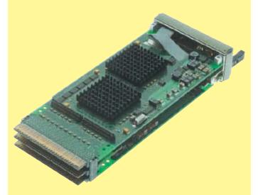
The MTCA.0 specification recommends the use of a special Plug Connector to reduce the insertion force of the module and to solve the tolerance stack-up problem between the multiple tongues and the backplane connectors.
