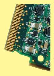
**PICMG** standard AMC.0 defines hard gold for the card edge interface. But a common and unique definition of hard gold does not exist today. As a result the quality of the gold pads in terms of hardness and roughness is highly unsteady. Additionally, the gaps between the pre and functional pad (which are necessary for the hot-swap ability) require a selective hard gold process which is
